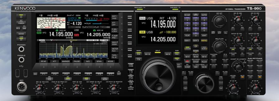
HF/50MHz Transceiver TS-990S Dual receiver & Dual TFT display
