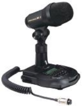
M-1 Reference microphone • Dual microphone configuration • Long stroke Smooth Operating PTT key • High visibility ON AIR LED • Nine-band graphic equalizer for each microphone element • Built-in record and playback feature
