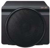
SP-30 High-Quality External Speaker • Speaker diameter: ø77mm • Maximum input: 12W • Impedance: 4Ω • Dimensions (W×H×D): (approx.) 4.5"×3.6"×10.4" (115×91×263mm) • Weight(approx.): 3.3 lbs (1.5kg)
