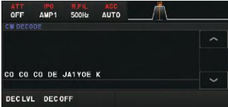
CW Decode display
