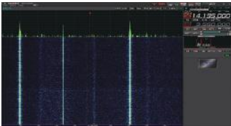
Band Scope (Waterfall) Display
