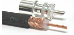
Properly prepare coaxial cable
