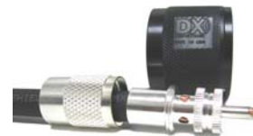
Remove tool and you're ready to solder
