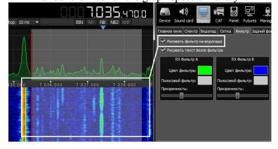
Render filter text - setting this check box include the display frequency filter settings and signal level in S-units within the filter used.
