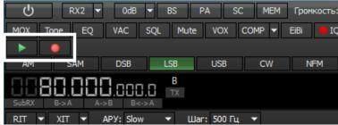
This function allows you to record the received audio signal. If necessary, the recorded signal can be retransmitted.
