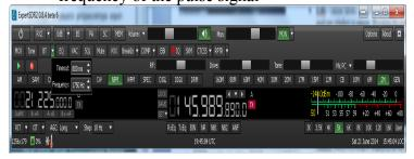
CTCSS – sub-audible tone squelch. Clicking the triangle, a drop down menu appears with a list of the standard sub-audible frequencies. Sub-audible squelch level is set at S-meter, as well as conventional squelch level.
