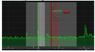
**XIT** - shifts your transmit frequency up or down while receive frequency does not change
