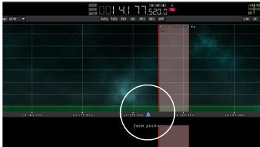
Regarding this center will be an increase. The triangle can be moved along the frequency scale in two ways thereby changing the frequency of which is increased relatively. Triangle can be moved by clicking the left mouse button can be clicked or frequency scale with the mouse wheel and the triangle will move instantly to a place clique.
