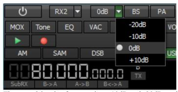
There are 2 levels of attenuation, -10dB and -20dB, and one level of pre-amp gain, 10dB.
