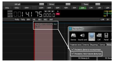
• Render S-Meter - setting the check box in this category includes an S-meter image near the receiver filter
