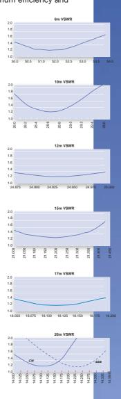
The R6000 employs quarter wavelength stubs on 10 and 15 meters to replace standard trap coils. The result is lower loss and wider bandwidth. The R6000 covers all bands 6 through 15 meters at a VSWR under 2:1. On 20 meters you can select the top 300 KHz or bottom 300 KHz of the band.
